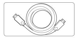
HDMI produces the best audio visual quality possible. Both audio and video signals are combined in one HDMI cable, providing an uncompressed, digital interface between your TV and HDMI devices. You must use HDMI to experience full high definition video. You must also use HDMI cables to use Philips EasyLink as described in Use Philips EasyLink on page 26.
